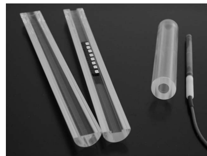
FIG. 1. Phantom A (right) for CTDI measurements with a pencil ionization chamber and phantom B (left) for dose measurements with OSLDs. Both phantoms had a diameter of 30 mm.
